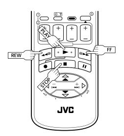
The easiest, most basic operation possible with your video recorder is tape playback. Already-recorded signals on a video tape are read by your video recorder and displayed on your TV just like a TV programme.
